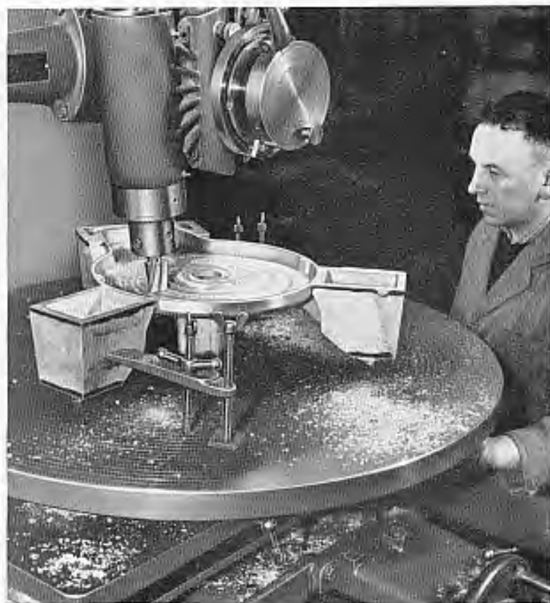
Recessing metal pattern for a hosiery machine head.
