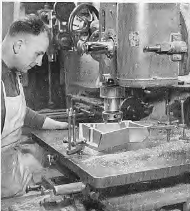
Surface milling using a 3½" diameter plug cutter cutterhead.
