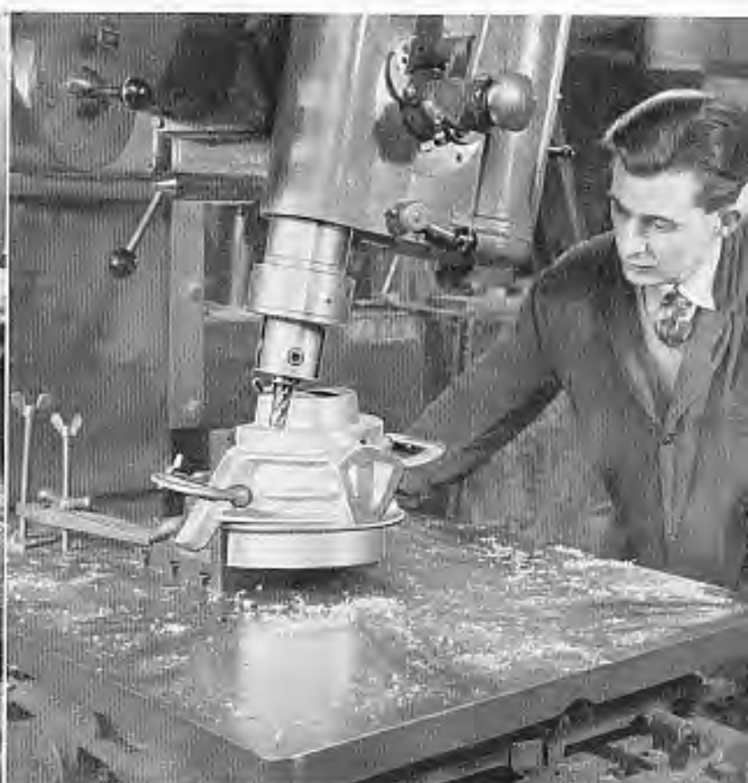
A wide range of milling cutters from ¼" to 2" diameter can be used on the machines. The four speeds on the spindle ensure correct cutting speed for each size of cutter.
