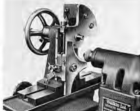
Fixture for regrinding semi-circular corebox cutters (item 1).
