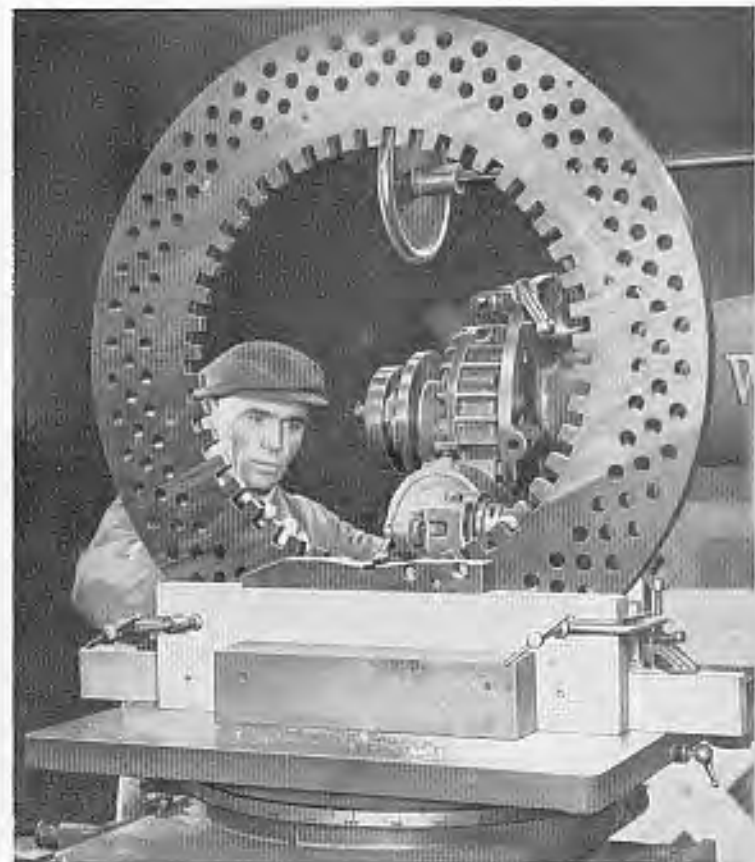
Machining a pattern ring in "PERMALI".
