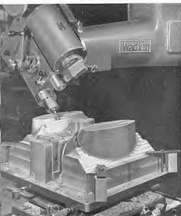
Machining aluminium air intake pattern on an aero engine pattern.
