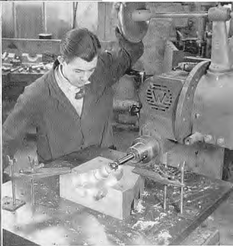
Machining an axle housing corebox, using a shortened cutter holder and tungsten carbide tipped cutter.
