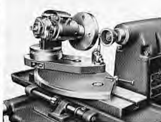
Fixture for regrinding face mills with inserted cutters.
