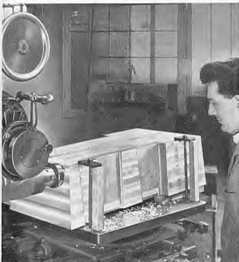
Milling an aluminum pattern for a machine base.
