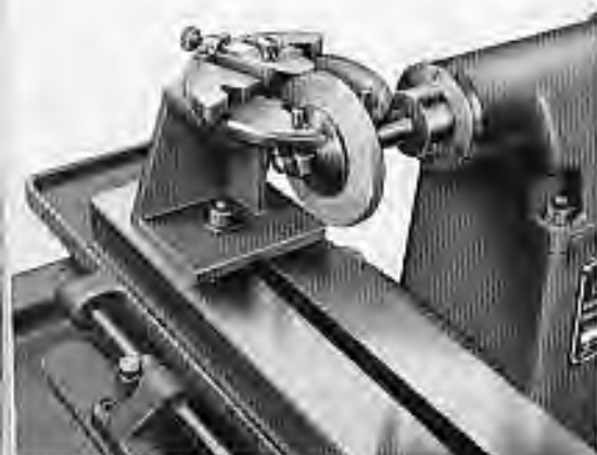
Fixture adapted for regrinding pattern cutters (item 2) using a formed wheel.
