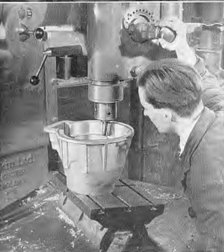
Milling inside a gear housing corebox.
