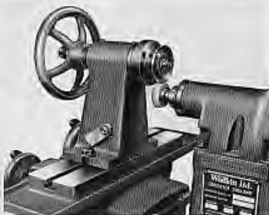
Regrinding clearance bevel on circular type corebox cutter (item 1a) using a formed wheel.
