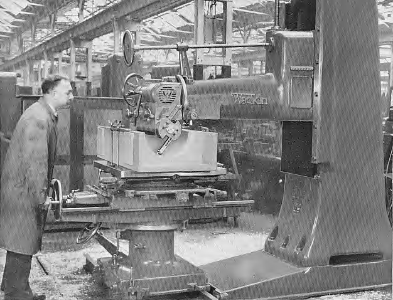
Machining inside corebox. This illustration demonstrates one of the big advantages of the latest model. The spindle is below the arm, which enables it to enter a corebox with its axis parallel with the face of the job. The cutterhead can be carried close up to the spindle bearing, and long bars and steadies are dispensed with.
