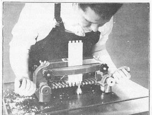
Dovetailing can be easily and efficiently performed on this machine.
