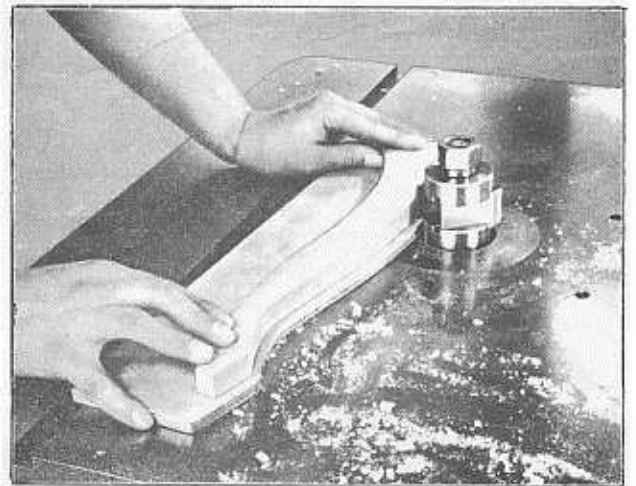
Shaping with slotted collars. (Universal guard removed to show detail).
