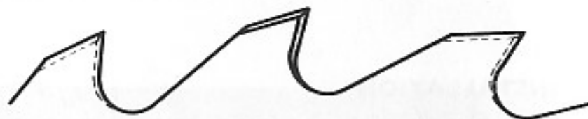
TOOTH PROFILE. STANDARD RIP SAW.
