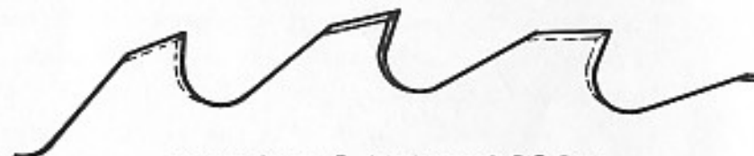
TOOTH PROFILE. THIN GAUGE RIP SAW.
