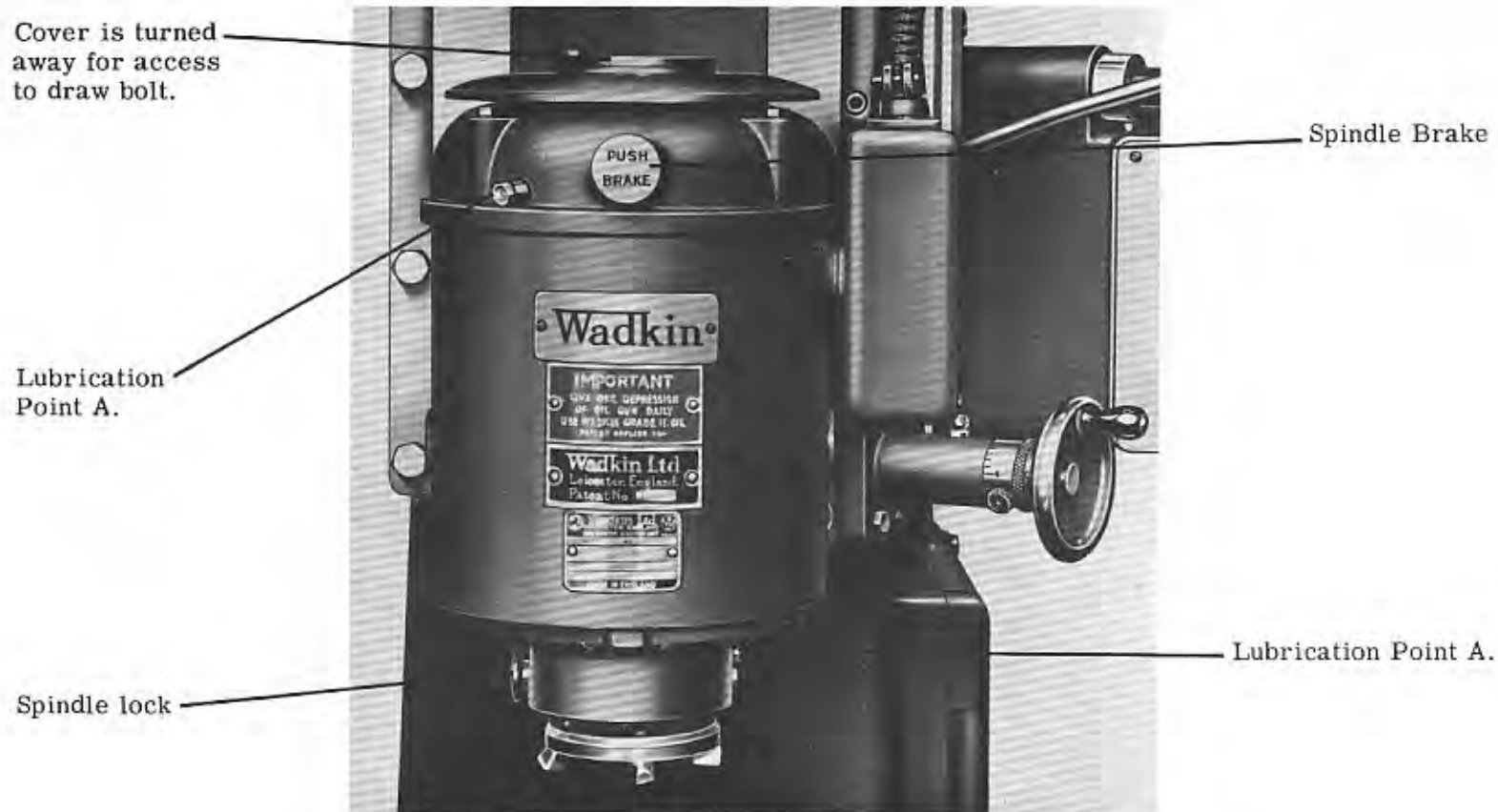
FIG. 3. VIEW OF ROUTER HEAD OF L. H. 1. MACHINE.
