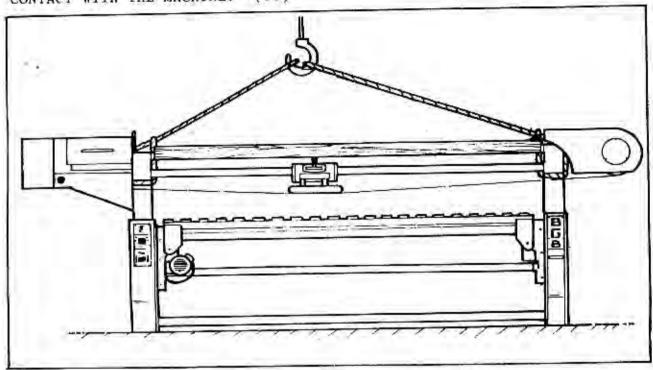
WHEN CRATED FOR EXPORT THE UNIT WILL WEIGH SOME 1200 kg, THE EXACT WEIGHTS, BOTH NETT AND GROSS BEING INDICATED ON THE CRATE. TO LIFT USE EVENLY SPACED SLINGS OR ROPES WHICH ARE KNOWN TO BE IN SOUND CONDITION. (ie)
